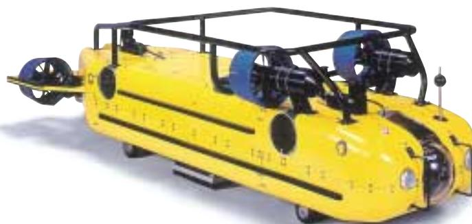
Thermal power station sluice inspection and cleaning robot
