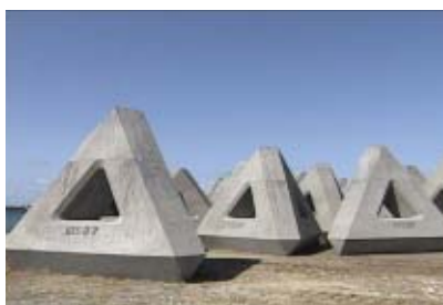
Breakwater blocks made of concrete incorporated with coal ash
