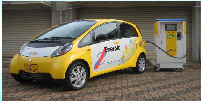
Mitsubishi Motors' i-Miev boosting charge equipment
