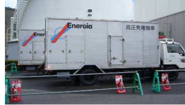
High-voltage generator vehicle (500 kVA, two vehicles)
