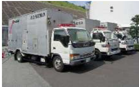
[ ] High-voltage generator vehicles
